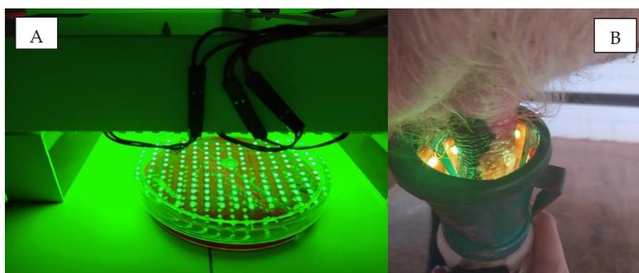
Figure 1. A) Green LED source ( $\lambda=520$  nm) with a light dose of 12.9 J/cm<sup>2</sup> for *in vitro* antimicrobial photodynamic therapy. B) Green LED light source ( $\lambda_{max} = 520$  nm, 12.7 mW/cm<sup>2</sup>) coupled to a conventional plastic teat for application of antimicrobial photodynamic therapy *in vivo*.
