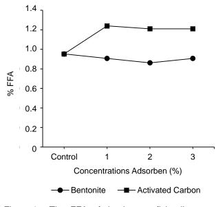
Figure 1. The FFA of the lemuru fish oil treated with bentonite and activated carbon
