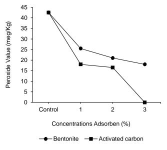
Figure 2. Peroxide value of the lemuru fish oil treated with bentonite and activated carbon
