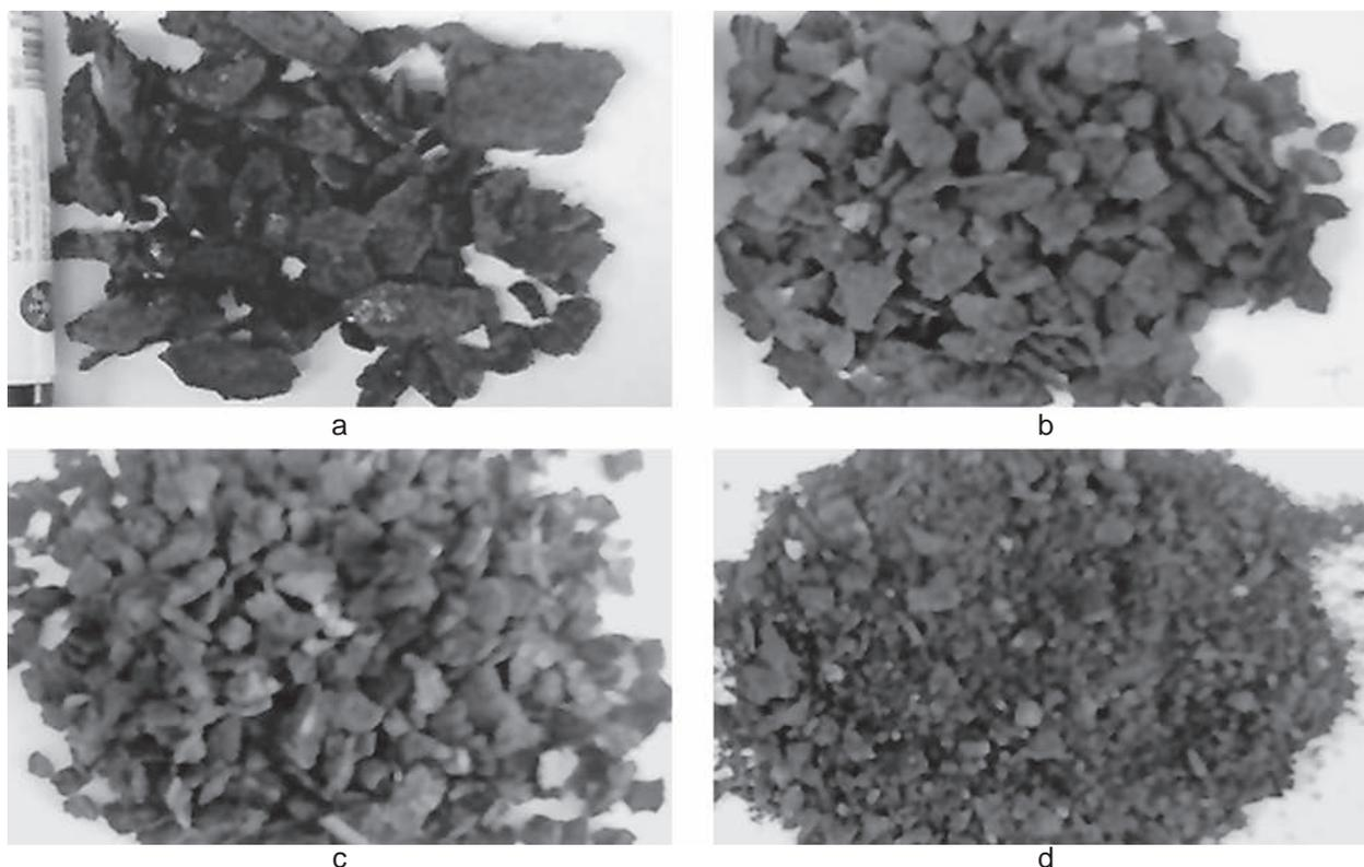
Figure 4. Sieving process result of compost based cacao pod at all grade level (Note: a = L grade size; b = M grade size; c = S grade size; d = SS grade size)
