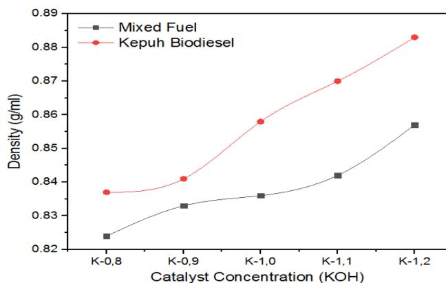
**Figure 3.** Graph of density relationship with catalyst concentration
