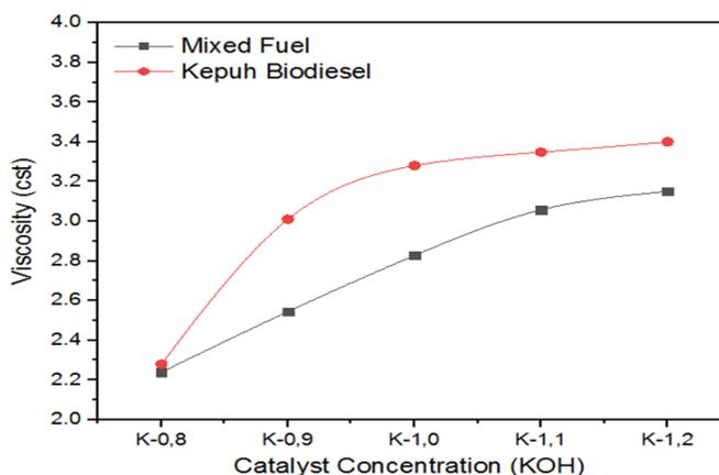
**Figure 4.** Graph of viscosity relationship with catalyst concentration
