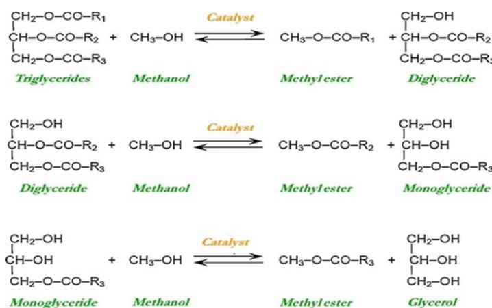
**Figure 2.** Transesterification reactions (Cercado et al., 2018)
