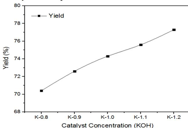
**Figure 6.** The relationship between catalyst concentration and steam. biodiesel yield
