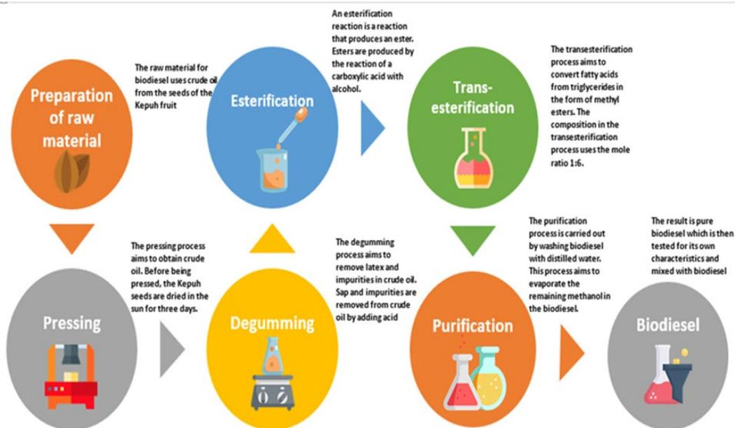
**Figure 1.** Biodiesel production process flow chart
