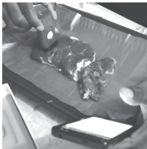
Figure 1. Spectra collection from fresh beef using a smartphone-assisted portable NIR spectrometer.
