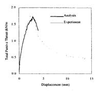
**Figure 7**. Analytical and experimental result for Toyoura sand
