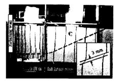
(w) is 3 mm for Toyoura sand and 9 mm for Soma sand. This result indicates that the thickness of shear band is known to be 20 times the mean particle diameter.
