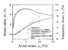
Figure 3. Simulated stress-strain volume of triaxial test
