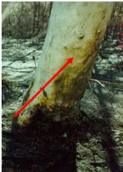
Figure 4 Angle of Char Fire Pattern Indicator on a tree trunk red arrow indicating the direction of the fire travel
