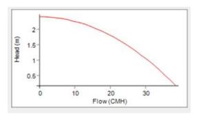
Figure 5. RAS system shrimp breeding infrastructure pump curve.
