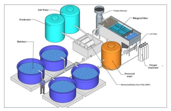
Figure 3. Recirculating aquaculture system shrimp breeding infrastructure placement scheme.
