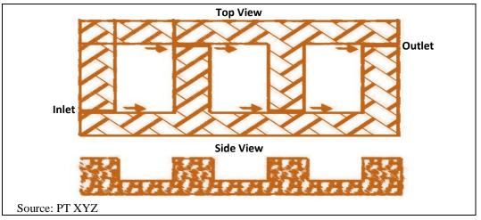
Figure 2 Settling pond design
