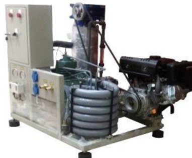
Figure 5 Innovation of slurry ice machine Indonesia using scraped-surface method with 500 kg/24 hours capacity operated with gasoline.
