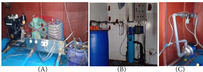
Figure 3 (A) Hot unit; (B) Cold unit; (C) Water system of slurry ice machine Indonesia operated with diesel oil on flat plate ship from KEMENRISTEKDIKTI RI at Politeknik Negeri Tual
