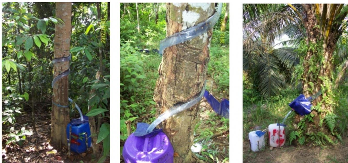
Figure 1 Setting up the measurement tool of stemflow volume.
