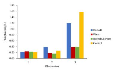
Figure 11. Phosphate content in aquaponic system with different filter treatments.
