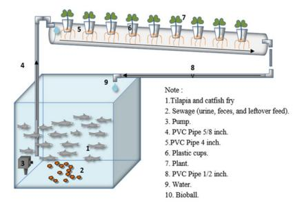
Figure 1. Recirculation system installation scheme
