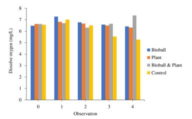
Figure 6. Dissolved oxygen content in an aquaponic system with different filter treatments.
