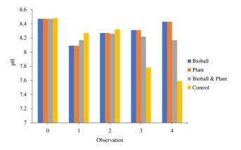
Figure 7. The pH value in aquaponic system with different filter treatments.
