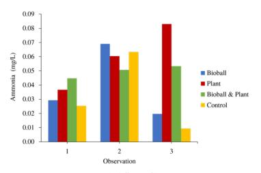
Figure 9. Ammonia content in aquaponic system with different filter treatments.
