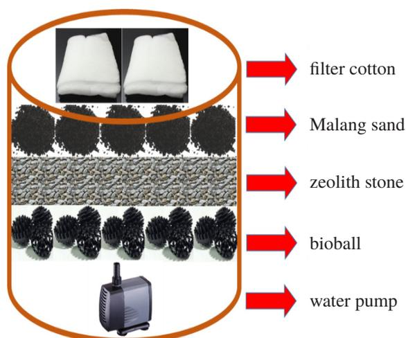
Figure 2. Filtering drum composition.
