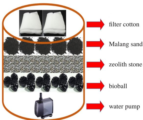
Figure 2. Filtering drum composition.
