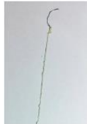
Figure 2. Several layers of spider silks were fixed to a suture needle
