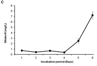
**Figure 1.** Rate of change of (A) ammonia-N, (B) nitrite-N and (C) nitrate-N during 5 days batch activity test. Values are given as mean  $\pm$  SE (n=3). SE = standard error.
