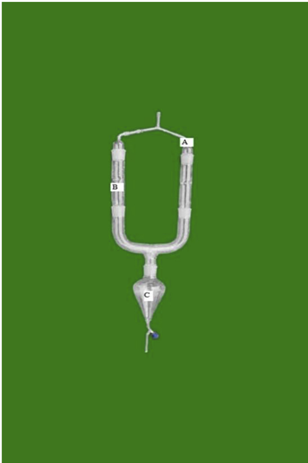
Figure 2. Olfactometer. (A) Y-tube. (B) Test chamber. (C) Release chamber.
