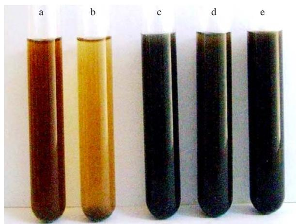
Figure 1. The color of compost extracts of vegetable wastes after being stored for 40 days. (a) Organic materials amended with *P. aeruginosa* Ch1 (B) without EM4 (E); [C-E+B]; (b) Organic materials with no amended either E or B, [C-E-B]; (c) Organic materials amended with E and B directly, then was extracted, [(C+E+B)] directly; (d) Organic materials amended with B and E, [C+E+B]; (e) Organic materials with E and without B, [C+E-B].
