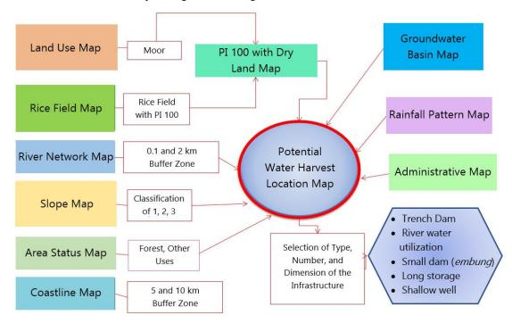
Figure 1. Diagram of the stages of determining the location and selecting the water harvesting infrastructure
