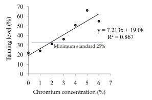
Figure 2. The correlation of chromium use with various levels of concentration and 8% concentration of gambier with the tanning level of tanned leather
