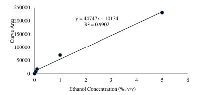
Figure 1. Standard curve of Ethanol
