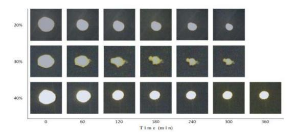
Figure 3. Gallery of images of a zedoary slice as a function of drying time at 20%, 30% and 40% RHs
