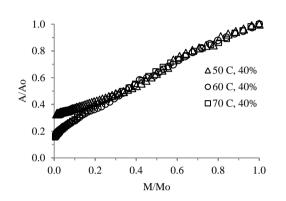
Figure 6. Dimensionless area changes  $(A/A_0)$  versus moisture content  $(M/M_0)$  at the different temperatures
