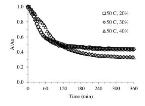
Figure 5. Area changes with drying time at the different relative humidities
