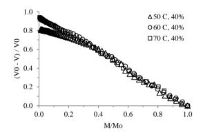
Figure 8. Total volume shrinkage  $((V_0-V)/V_0)$  versus moisture content  $(M/M_0)$
