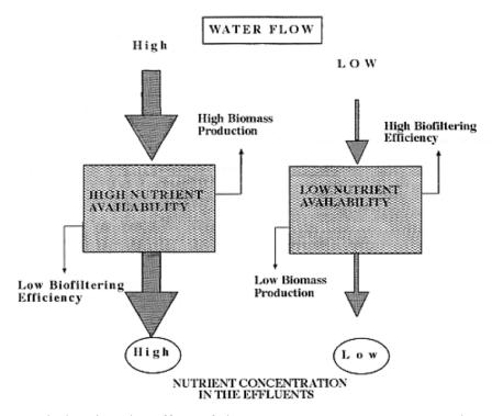
Figure 7. General showing the effect of the water turnover rate on growth and biofiltering efficiency (Buschman *et al.*, 2001).
